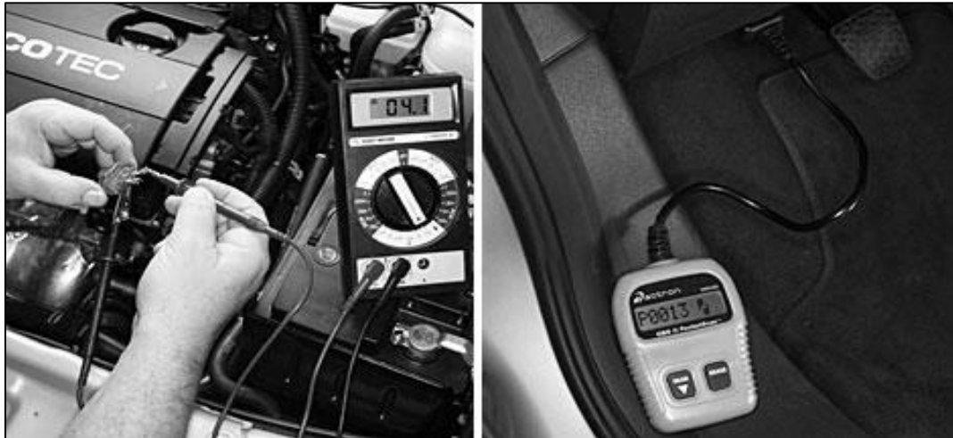
RAJAH 11 : TEST SENSOR USING MULTIMETER
