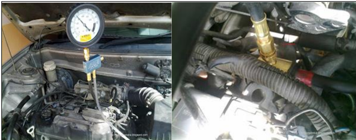
RAJAH 4: PEMASANGAN PRESSURE TESTER
