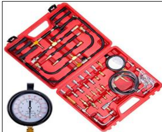
RAJAH 3 : FUEL PRESSURE TESTER TOOLS
