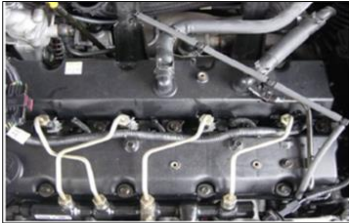
RAJAH 3 : HIGH PRESSURE DELIVERY PIPE
