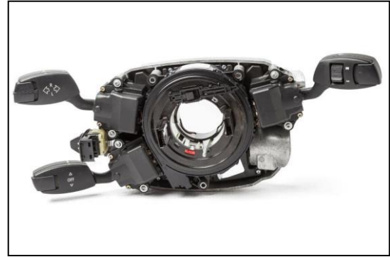
RAJAH 6 : STEERENG ANGLE SENSOR / POSITION SENSOR
